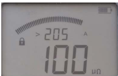
Min current during test was 205 A
