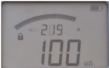
Max current during test was 219 A.
