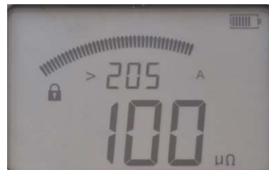
Pictures shows that the test current was below 219 A and over 205 A.
