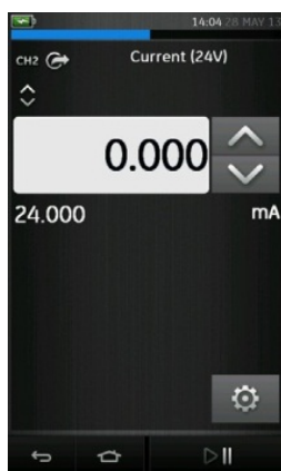
Figure 2-18 Source current on CH2 with internal loop power. (Range: 0 to 24\text{mA} )
