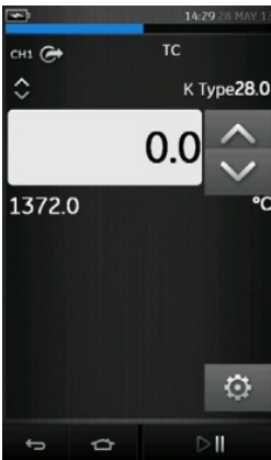
Figure 2-25 K-Type Thermocouple Source CH1 (Range -270 to 1372 °C)
