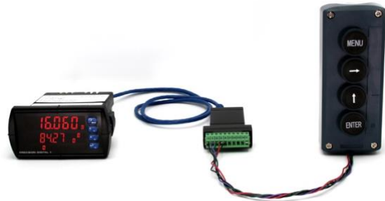
Figure 26. Meter to Control Station Connection
