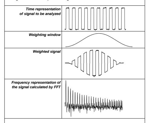
The total duration of the study interval results in a convolution in the frequency domain of the signal with a function sinx/x.
