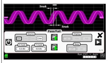
When a value is entered, the message "mask calculation in progress" appears, then the new mask is displayed
