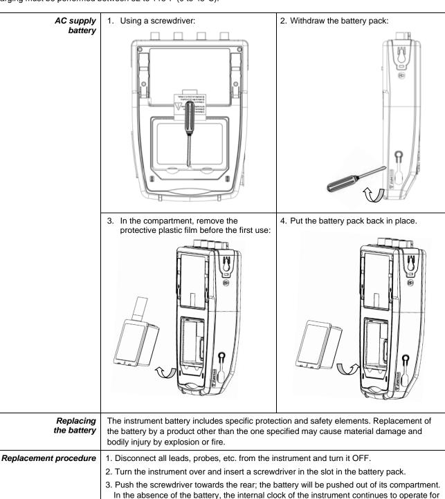
4. Insert the new pack in the compartment and press it firmly in place.
