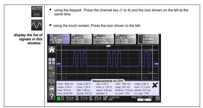
To start Auto measurements in the 4 channels:
