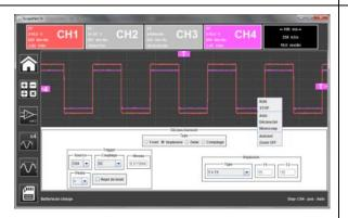
In Oscilloscope mode, ScopeNet IV proposes adjustments by a right click on the waveform: RUN/STOP, AUTO/TRIG/SINGLE/AUTOSET and ZOOM are easy-to-configure parameters.
