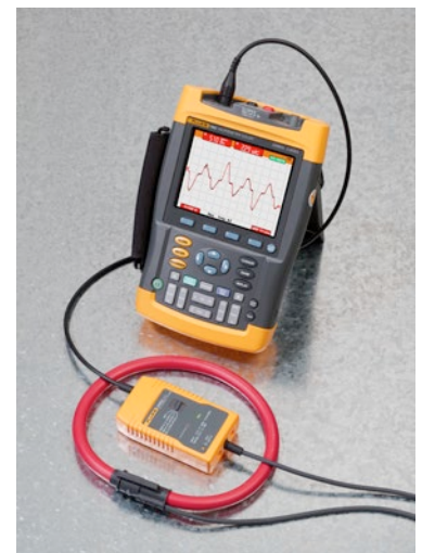
i3000s Flex connected to a Fluke 199C ScopeMeter.
